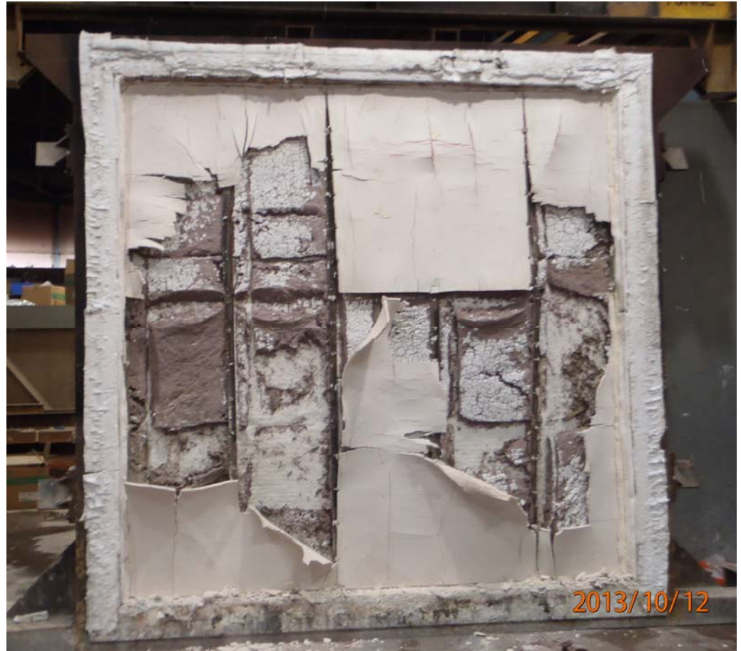
The exposed face of the specimen shortly after the test and just before the hose stream test
