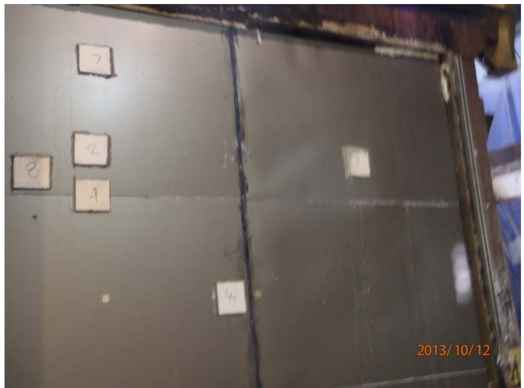
The unexposed face of the specimen during the hose stream test
